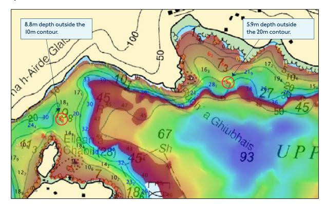
This example demonstrates how using a colour banded sounding selection helps to identify depths of interest.
