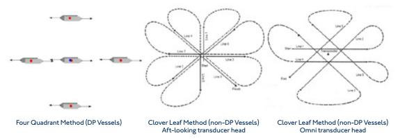
Alternative patterns for non-DP vessels include navigating the vessel in a circle centred on the transducer position, potentially followed by the four-quadrant method with the vessel held as stationary as possible using manual control of propulsion and thrusters. These patterns should be used if specified for the USBL calibration utility in use.
