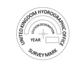
The marker and all installation equipment must be provided by the Company and engraved as illustrated above
