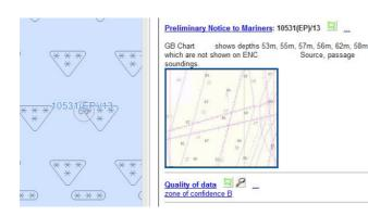
The full text of the NM can be viewed in the ECDIS Pick Report. Where additional information is needed to explain the NM an associated picture file displays the ENC superimposed over the current paper chart information.
